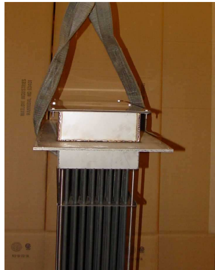
Figure 4 - For Vertical lifting place strap through the space between the element bundle and the insulation retainer. Do not slip the strap through the elements.
